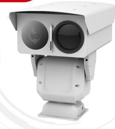
Hikvision DS-2TD8166-100C2F/V2 Thermal & Optical Bi-spectrum Network Stable PTZ Camera equipped with built-in GPU which support intelligent behavior analysis algorithm, can realize high precision VCA detection and real-time alarm. It is applied to frontier defense occasions, maritime defense occasions, port monitoring, airport perimeter security, and so on. The pre-alarm system helps you discover unexpected events immediately and protects you from property loss.
